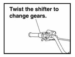
When starting and going up hills, use the 1<sup>st</sup> gear. When pedaling at higher speeds, use the 2<sup>nd</sup> and 3<sup>rd</sup> gears. Changing gears does not require that the bike be powered by the battery. The gear shifting system and motor are entirely separate and neither affects the other's performance. Both work toward the goal of propelling the bike, of course, and their contributions are additive.
